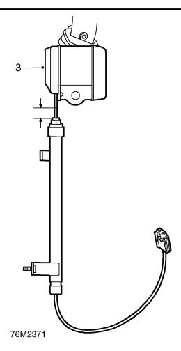
**3.** Remove reel from gas generator by cutting flexible link approximately 10 mm from end of gas generator tube.
