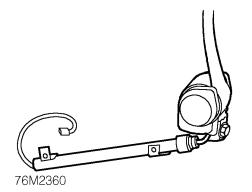
The front seat belt reels are linked by cables to gas generators housed within remote steel tubes. The generators are driven by small quantities of nitrocellulose. On receiving a fire signal from the DCU, the generators deploy to force pistons down the steel tubes, pulling the cables tight. The cables are connected to the seat belt reels which in turn pull the seat belts tight, reducing any slack in the belts.
