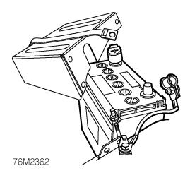
• Always disconnect both battery leads, earth lead first before commencing work.
