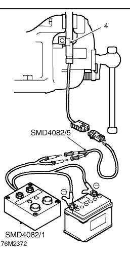
4. Position gas generator tube vertically in vice with fly lead at bottom and tube bracket positioned on vice side to prevent tube being forced out of vice. Tighten vice to hold tube rigid and secure. DO NOT OVERTIGHTEN.
