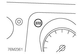
The SRS warning lamp, located on the fascia, illuminates when the electrical circuits are switched on whilst the system performs a self diagnosis test. If the system finds no fault during self diagnosis the light will extinguish after approximately 5 seconds and remain extinguished.
