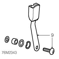
**9.** Remove Torx screw securing seat belt stalk and remove stalk.
