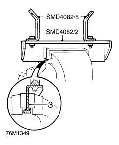
**3.** Position tool **SMD 4082/2** in vice, ensuring that vice jaws grip tool above bottom flange to prevent possibility of tool being forced upwards from vice. Tighten vice.
